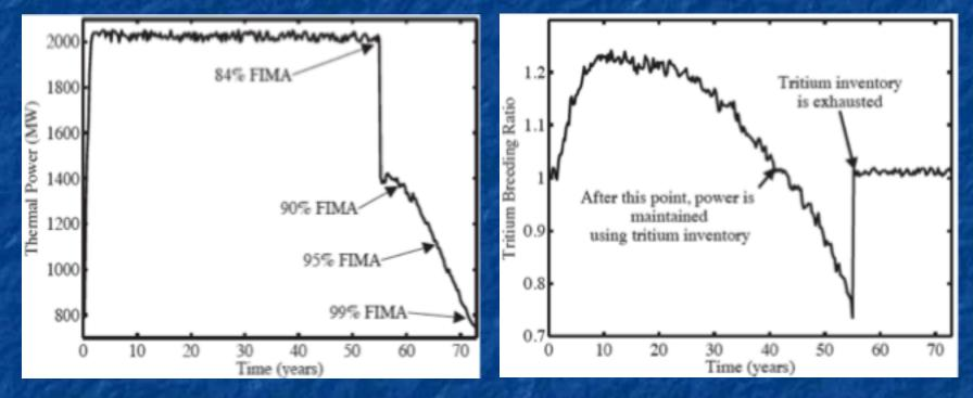
"This design produces 2000 MWt of power for over 50 years using a fuel loading of 40 MT. Fuel enrichment and reprocessing are not required. Early results show promise for this system with limitations being driven by self-sufficient tritium production."<sup>3</sup>
