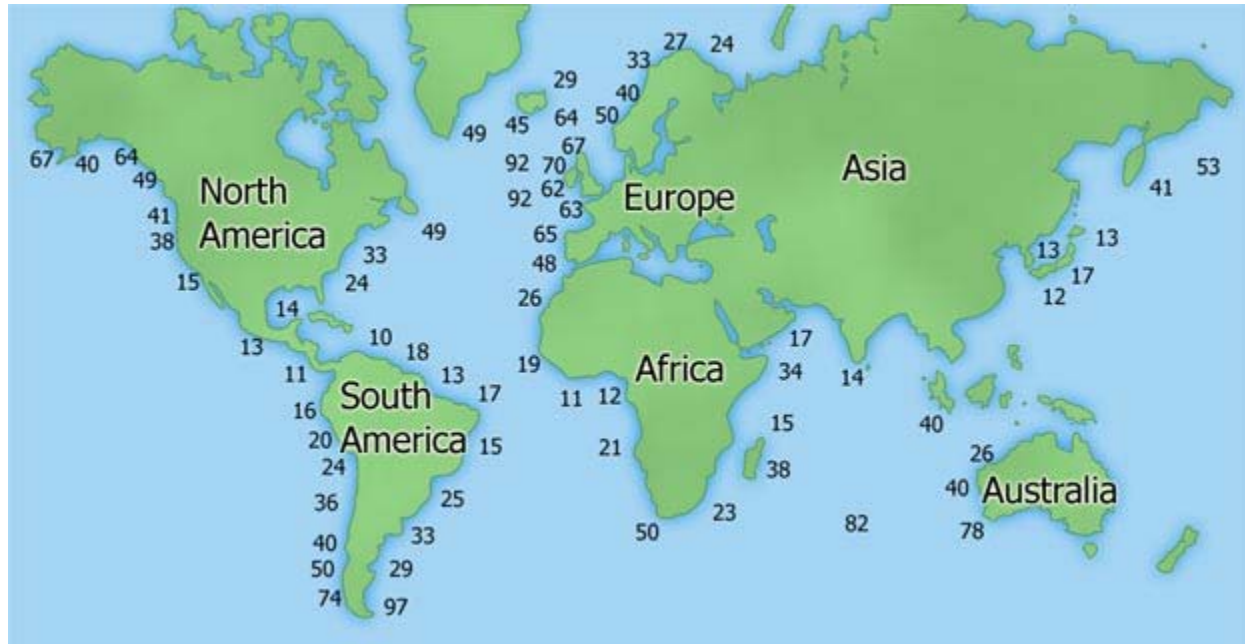
Figure 9: This map shows the average energy for waves along coastlines. The values given are in kW per meter of wave.
