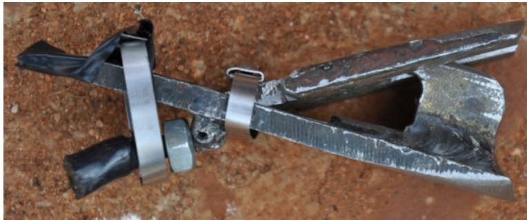
Figure 7: The Harpoon of Death, up close. A link of chain slips around the hook at the right, and the edge at the extreme lower right is sharpened to grab the bottom of a pipe segment inside a coupling. [June 17]
