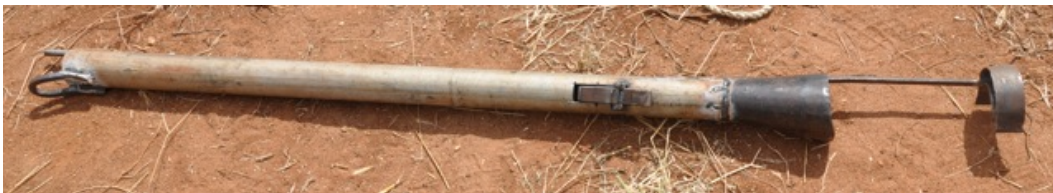
Figure 10: The Rocket of Reclamation, which was initially welded in Wote on 21 June 2010. The curved structure at the right is the “scythe” designed to sweep the pipe away from the wall and into the Rocket’s funnel.
