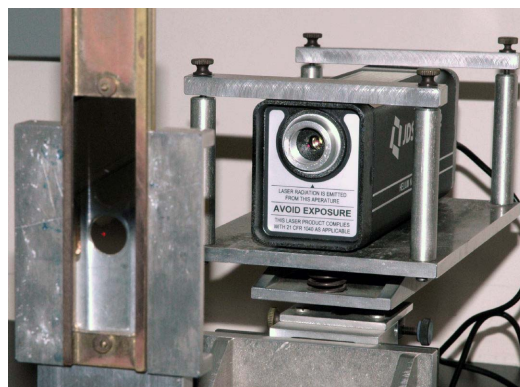
Figure 5.8 The attenuator is the partially silvered glass slide at the left. Note the small red dot of the helium-neon laser beam, which has a wavelength of 632.8 nm.
