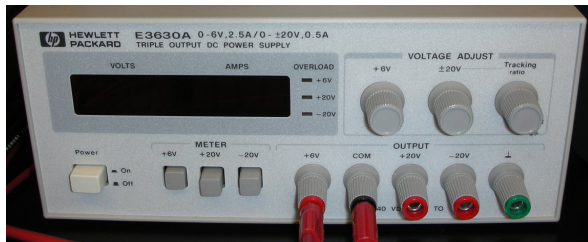
Figure 1.5 A DC power supply. Use the 6-V output port and the common.
