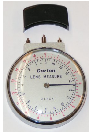
Figure 4.13 The diopter gauge, which allows you to measure the refractive power of a glass lens surface. It works by placing three round-ended rods against the lens surface. The two outer rods are fixed; the central one is spring loaded and operates the dial of the gauge. The black object is a cap to protect the rods. Please keep the gauge capped when you are not using it to measure a lens surface.
