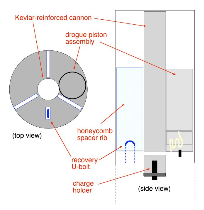
2) Detail view of lower payload section with structural and mounting members
