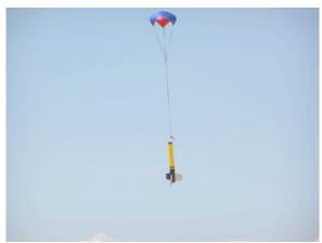
(d) main deployment fouled by piston strap
