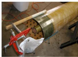
(i) application of carbon/Kevlar reinforcement band to upper midbody airframe
