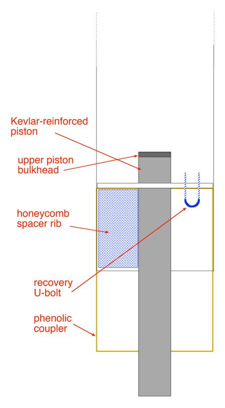
Photos documenting construction details and hidden interior components (for more photos and details, see <u>http://www.physics.hmc.edu/GL/WAC/gindex.html</u>):
