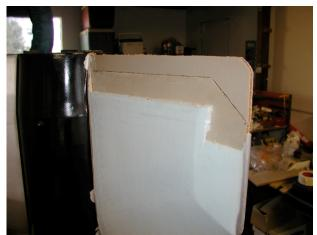
(c) replacement of crushed fin edge
