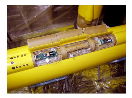
The wires for the matches reach the compartments via pass-through holes from the recovery bays. Switch and shunt wiring pass along the sides of the compartments as shown in the detailed views below.
