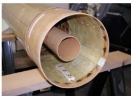
(e) internal view of reinforced joint coupler with compression bar
