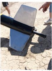
(f) fin damage due to hard landing
