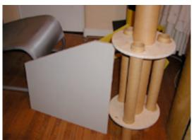
(a) motor mount assembly with fin core
