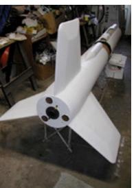
(k) rear view of complete lower and midbody sections with primer applied
