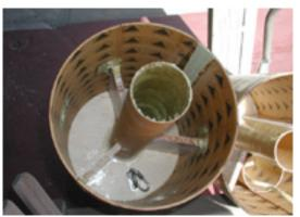
(h) internal view of payload ejection piston with bulkhead and hardware
