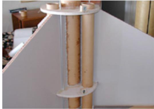
(b) fins glued and filleted to motor mounts
