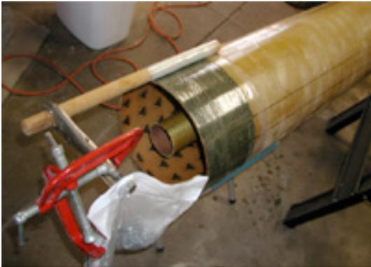
(i) application of carbon/Kevlar reinforcement band to upper midbody airframe
