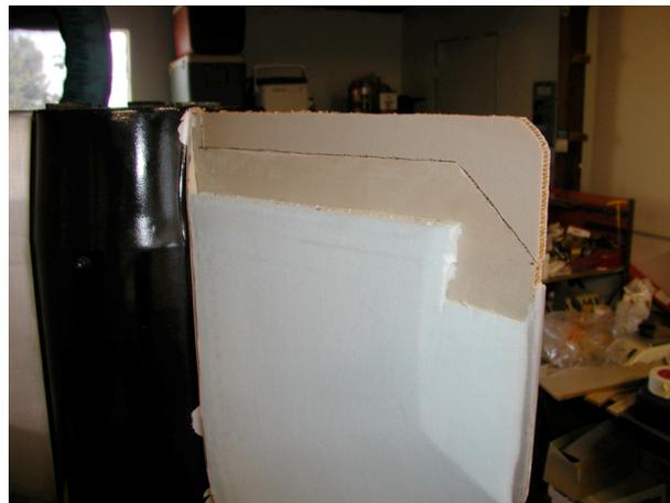
(c) replacement of crushed fin edge
