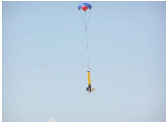
(d) main deployment fouled by piston strap
