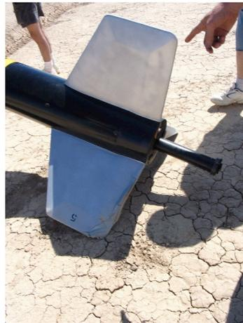
(f) fin damage due to hard landing
