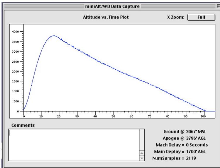
seconds later, the drogue piston fired and deployed the drogue chute. The drogue inflated and relatively gently reoriented the falling booster from nose-first to tail-first descent.
