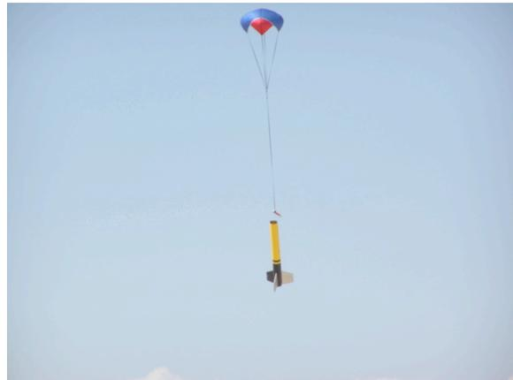
(d) main deployment fouled by piston strap
