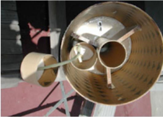
(g) internal view of midbody recovery bay with drogue piston, U-bolt and ribs
