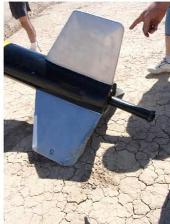
(f) fin damage due to hard landing
