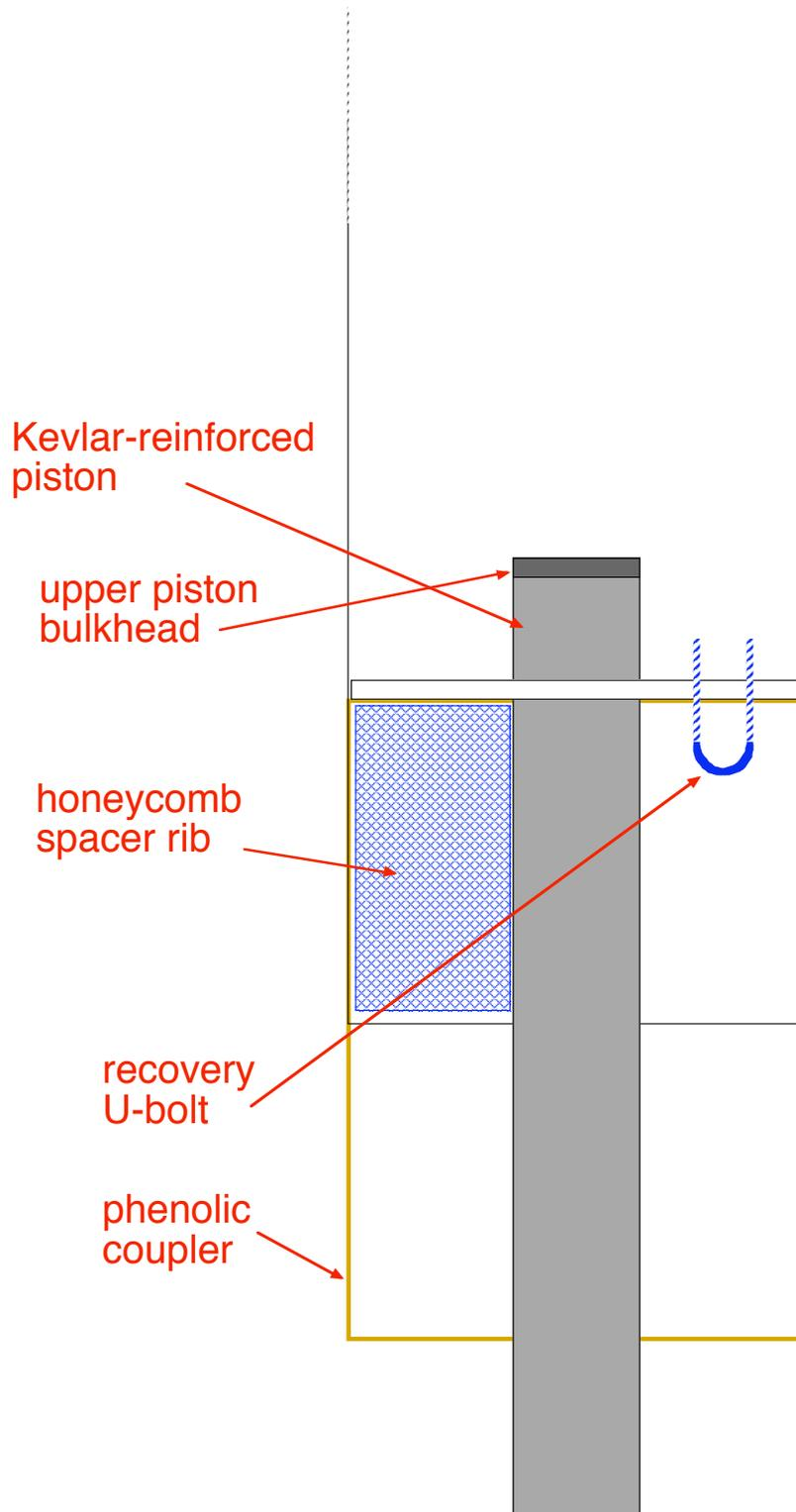
Photos documenting construction details and hidden interior components (for more photos and details, see <http://www.physics.hmc.edu/GL/WAC/gindex.html>):
