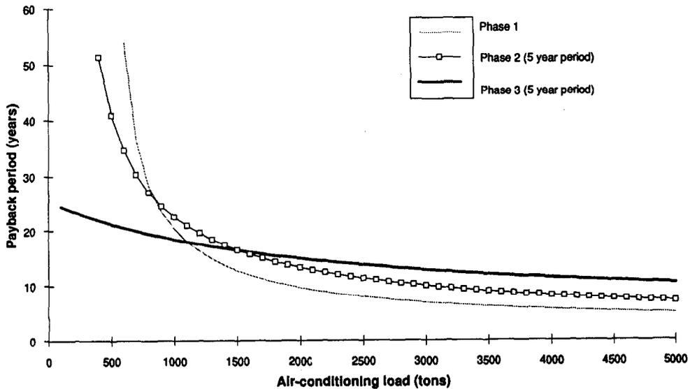
Fig. 6a. Payback period as a function of air-conditioning load for the sample OTEC plant project (20  $\epsilon$ /kWh electricity, 5-year phase spacing).
