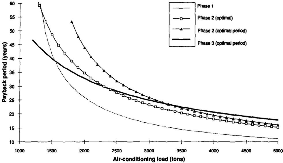
Fig. 5. Payback period as a function of air-conditioning load for the sample OTEC plant project (10  $\epsilon$ /kWh electricity).
