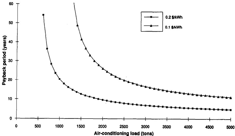
Fig. 1. Payback period as a function of air-conditioning load for Phase 1 of a sample OTEC plant project utilizing a 1.6 m diameter CWP.
