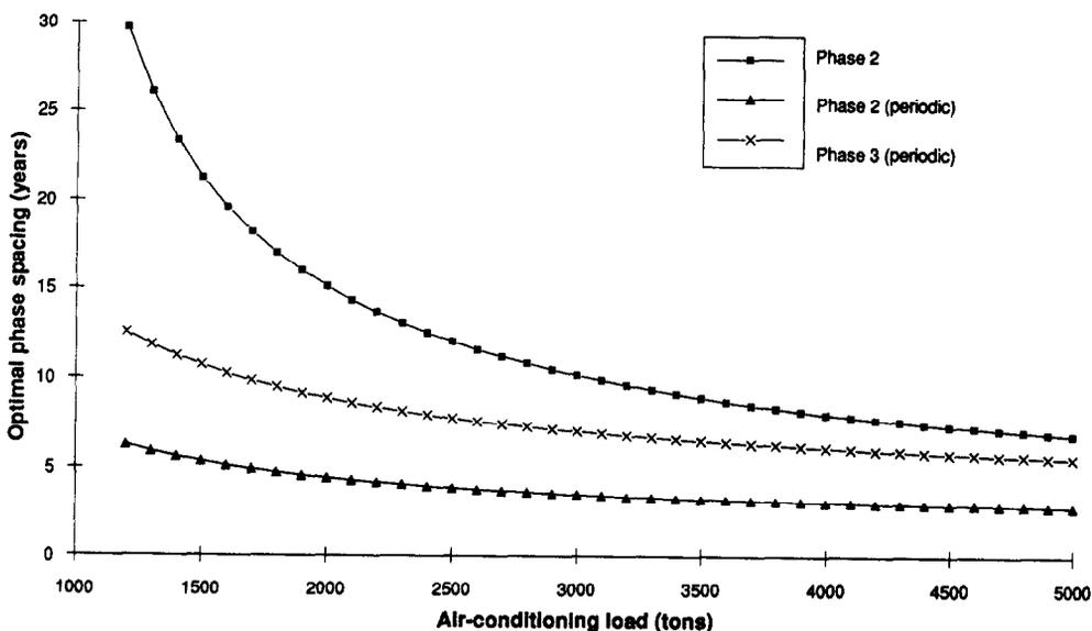
Fig. 4. Optimal phase spacings for a two-phase or three-phase-periodic implementation of the sample OTEC plant project (10 ¢/kWh electricity).
