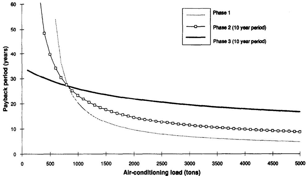
Fig. 6b. Payback period as a function of air-conditioning load for the sample OTEC plant project (20 ¢/kWh electricity, 10-year phase spacing).
